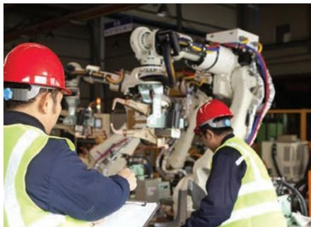
Often called Third-Party Inspection or Source Inspection, Vendor Inspection covers activities performed at manufacturer's work. This includes all types of electronic, mechanical, instrumentation, and electrical equipment bought for the Oil and Gas, Mining, Pharmaceutical, and Petrochemical industries.
